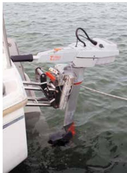
We mounted the three different types of engines on a Catalina 22 to compare them. Speed data was collected with a GPS while steering reciprocal courses at slack tide. From left: 5-horsepower Lehr, 5-horsepower Mercury SailPower, and the Torqeedo Travel 1003.
